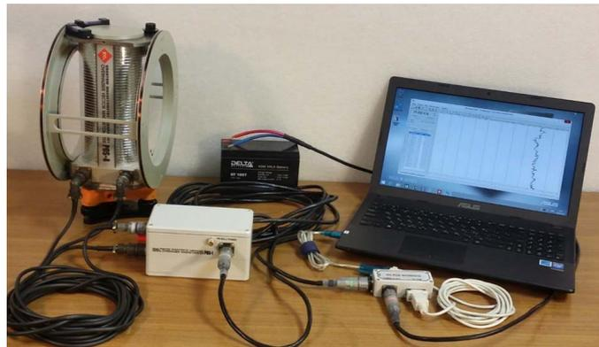
**Figure 6.** Vector/scalar Overhauser DNP magnetometer POS-4.
