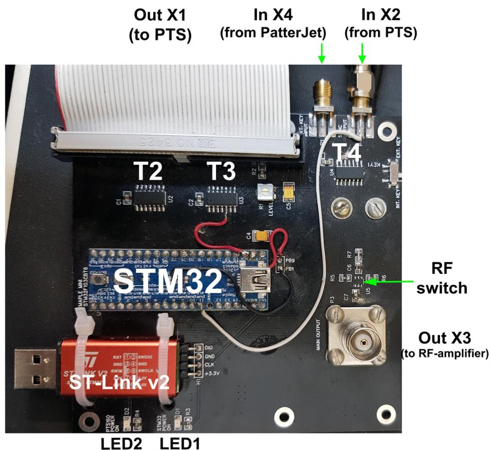
**Figure 3.** Picture of designed control board U1 for RF pulses generation with highlighted the main parts. T2–T4 are TTL forming units.
