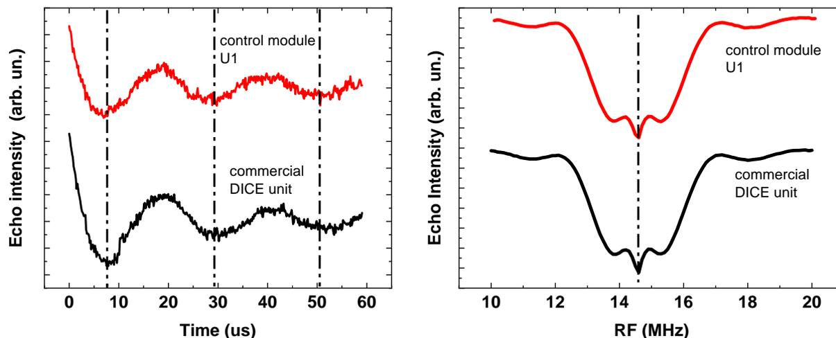
**Figure 4.** Implementation of X-band Mims-ENDOR. The signals obtained with the developed control module U1 are highlighted in red, the signals obtained with the commercial DICE ENDOR unit (Bruker, Germany) are highlighted in black. (a) Nutation experiment at RF of 14.6 MHz. (b) Dependence of the electron spin echo on the frequency of the RF pulse.
