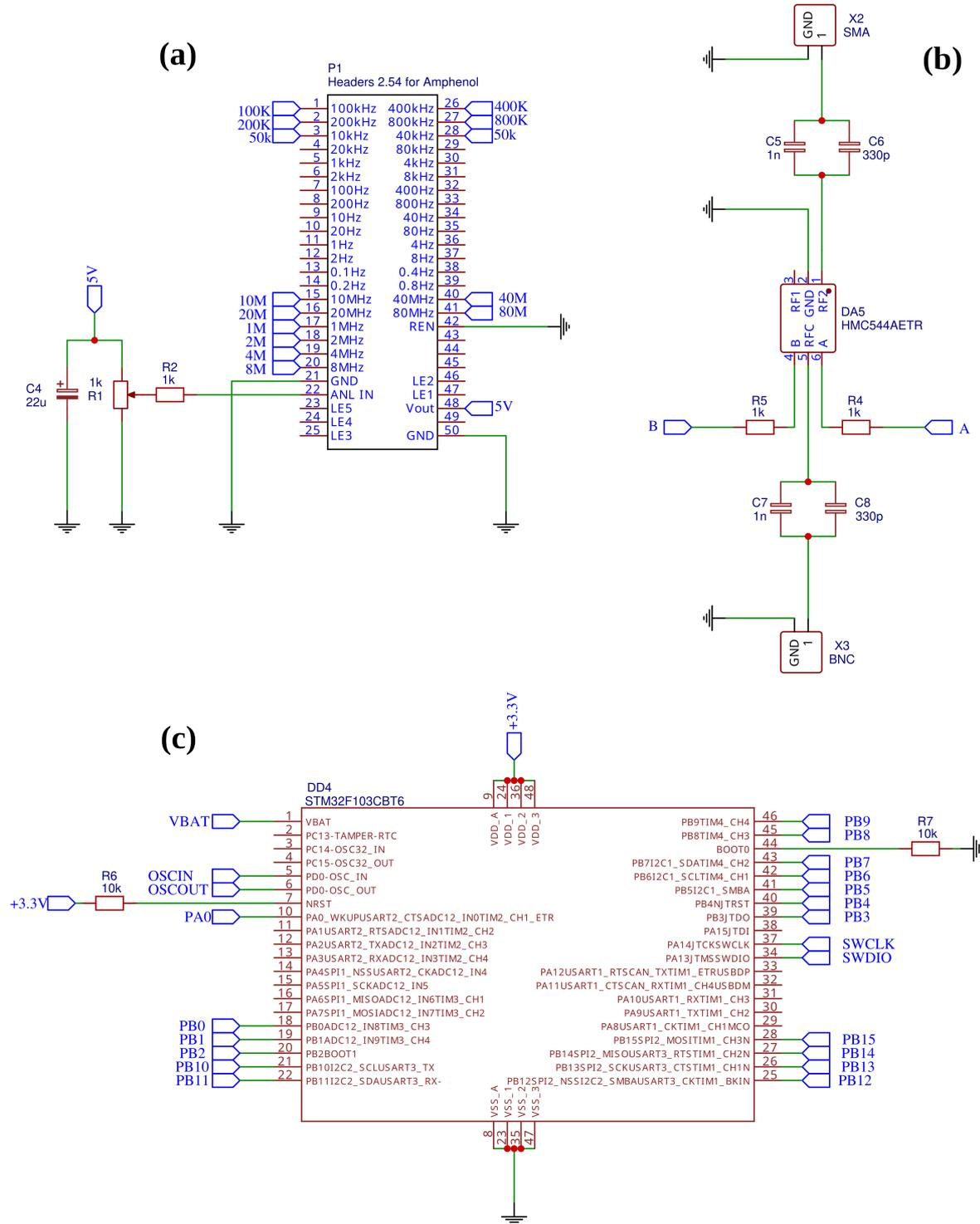
**Figure 2.** Electrical circuits of the control module. (a) TTL register diagram for the PTS input to generate harmonic signal with a specific frequency. (b) Scheme for creating RF pulse using a SPTD (Single Pole Double Throw) switch HMC544AETR (DA5). (c) Diagram of the STM32F103CBT6 pins involved.
