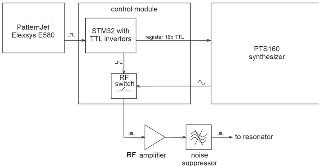
**Figure 1.** Implementation scheme for RF control.
