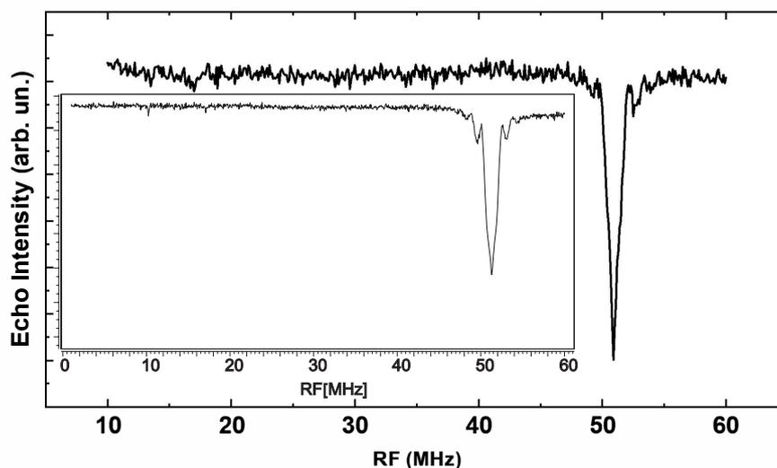
**Figure 5.** Q-band Mims-ENDOR spectra of coal obtained using developed control module. In inset the spectrum adopted from the Bruker user’s manual (see Fig. 4–5 on page 4–8 in Ref. [15]).
