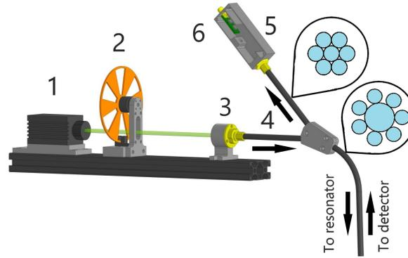
**Figure 1.** Optical part of the ODMR attachment. (1) A 532 nm diode-pumped laser, (2) an optical obturator, (3) 1064 nm filter and collimator, (4) optical fiber 400  $\mu\text{m}$ , (5) silicon photodiode, (6) preamplifier.
