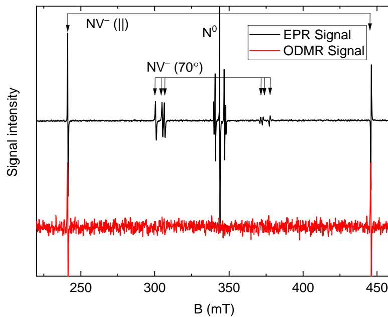
**Figure 2.** EPR (black, top) and ODMR (red, bottom) spectra of single-crystal diamond samples activated by paramagnetic  $NV^-$  centers in the orientation [111].
