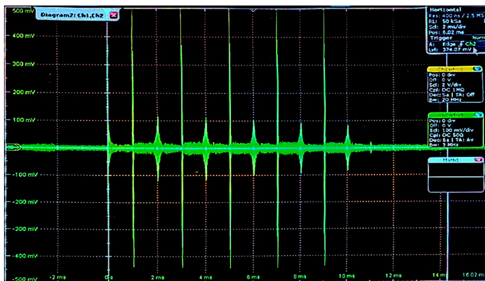
Figure 7. Receiver output signal during the action of generated Carr-Purcell-Meiboom-Gill (CPMG) pulse sequence
