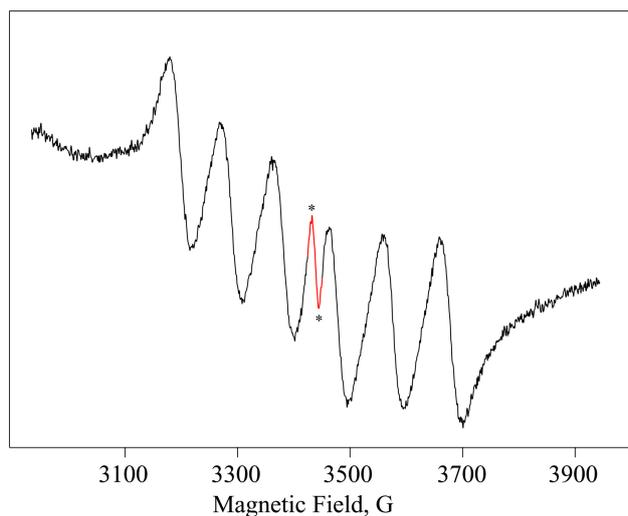
**Figure 3.** The EPR spectrum recodered for leaves material (control). The additional line is indicated by the asterisks symbols.
