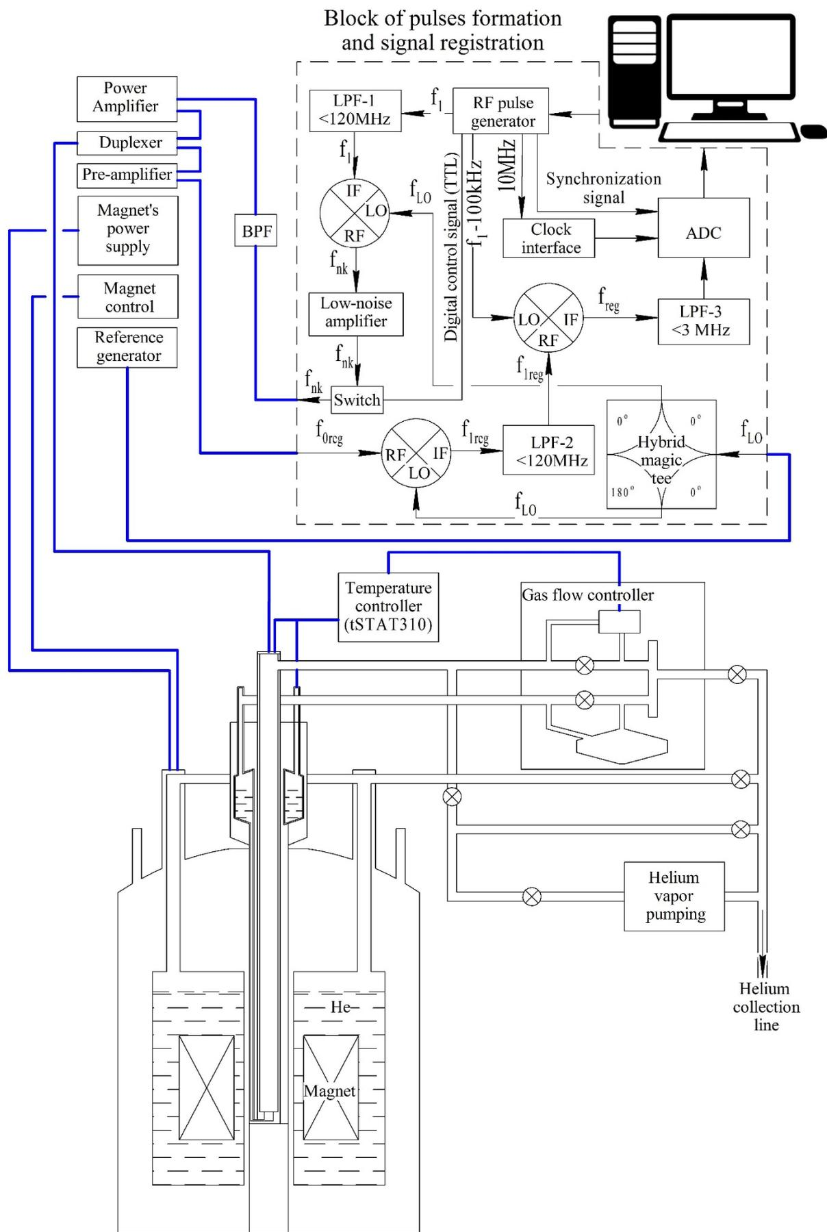
Figure 1. Block diagram of the pulsed NMR spectrometer.
