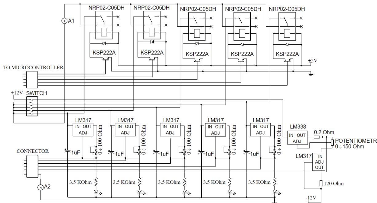
**Figure 3.** The scheme of the magnet control.
