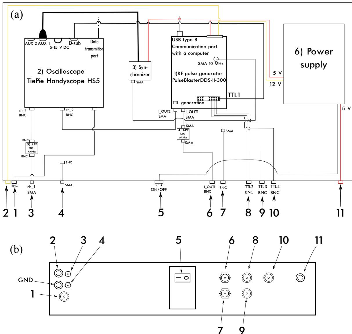
**Figure 1.** (a) Block diagram of the transmit-receive path. (b) An image of the front panel of the transmit-receive path. The numbers indicate the following parts:
