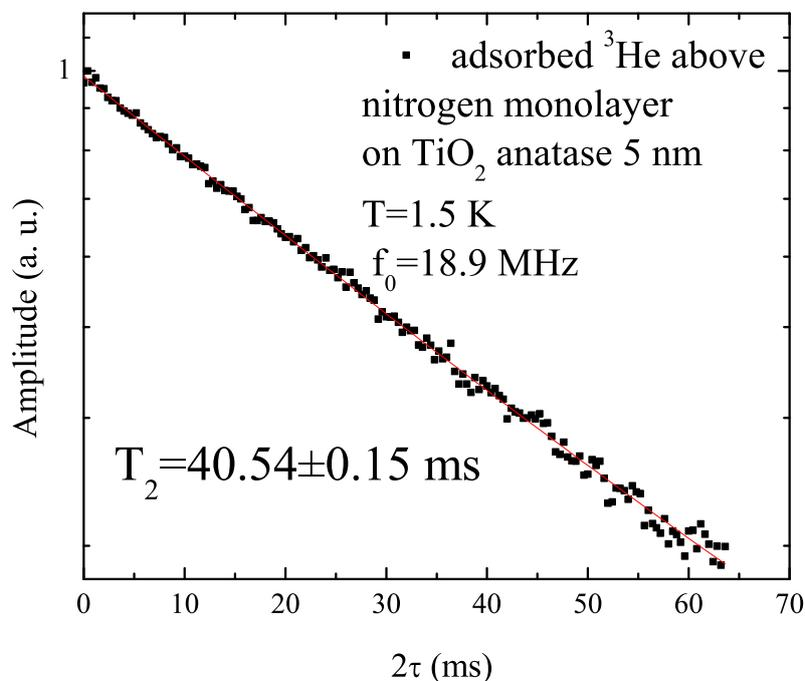
Figure 7. The example of the transverse magnetization decay of  $^3\text{He}$  nuclei received by CPMG sequence application to adsorbed  $^3\text{He}$  above nitrogen monolayer in contact with  $\text{TiO}_2$  nanopowder at 1.5 K and 18.9 MHz.
