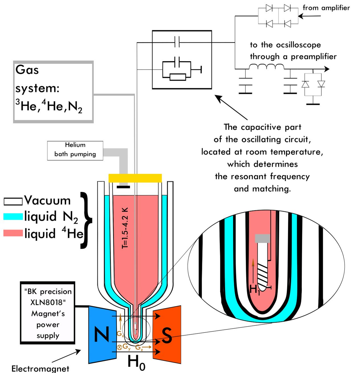
Figure 5. Block-scheme of glass cryostat, magnet and gas system.
