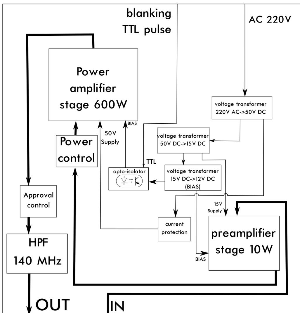
Figure 2. Block-diagram of pulsed amplifier used in the spectrometer.
